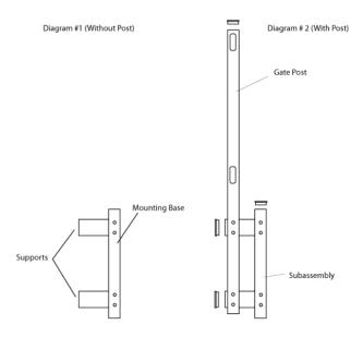
The maximum width of the gate is 38". If you do not have two uprights positioned within that measurement, use an artificial upright for one of the gate posts.
